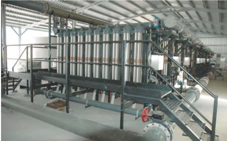
Electrowinning plant with cells for producing silver powder.
